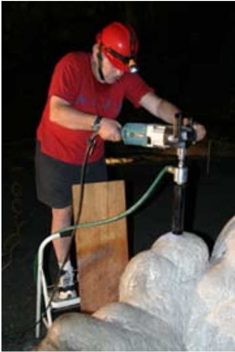
Coring a stalagmite in August 2008 using a newly designed corer.
